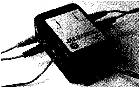
TO RECORD FROM A TURNTABLE to your Mac, you need to use a phono preamp like the one shown here.
